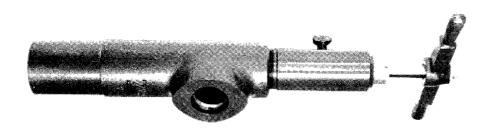
TECTROL has been manufacturing a long nose gas choke for several years. We were the first in the industry to build a 7800 PSIG choke that conformed to the American Petroleum Institute 1984 Specification 12K (June 20, 1984). Each choke is pressure tested at our factory to one and one half (1½) times working pressure or 11,700 PSIG. We have a saying at TECTROL, "If it's painted, it's tested."
