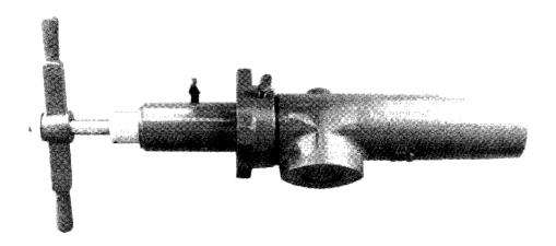
TECTROL has been manufacturing a long nose gas choke for several years. We were the first in the industry to build a 7800 PSIG choke that conformed to the American Petroleum Institute 1984 Specification 12K (June 20, 1984). Each choke is pressure tested at our factory to one and one half (1½) times working pressure or 11,700 PSIG. We have a saying at TECTROL, "If it's painted, it's tested."
